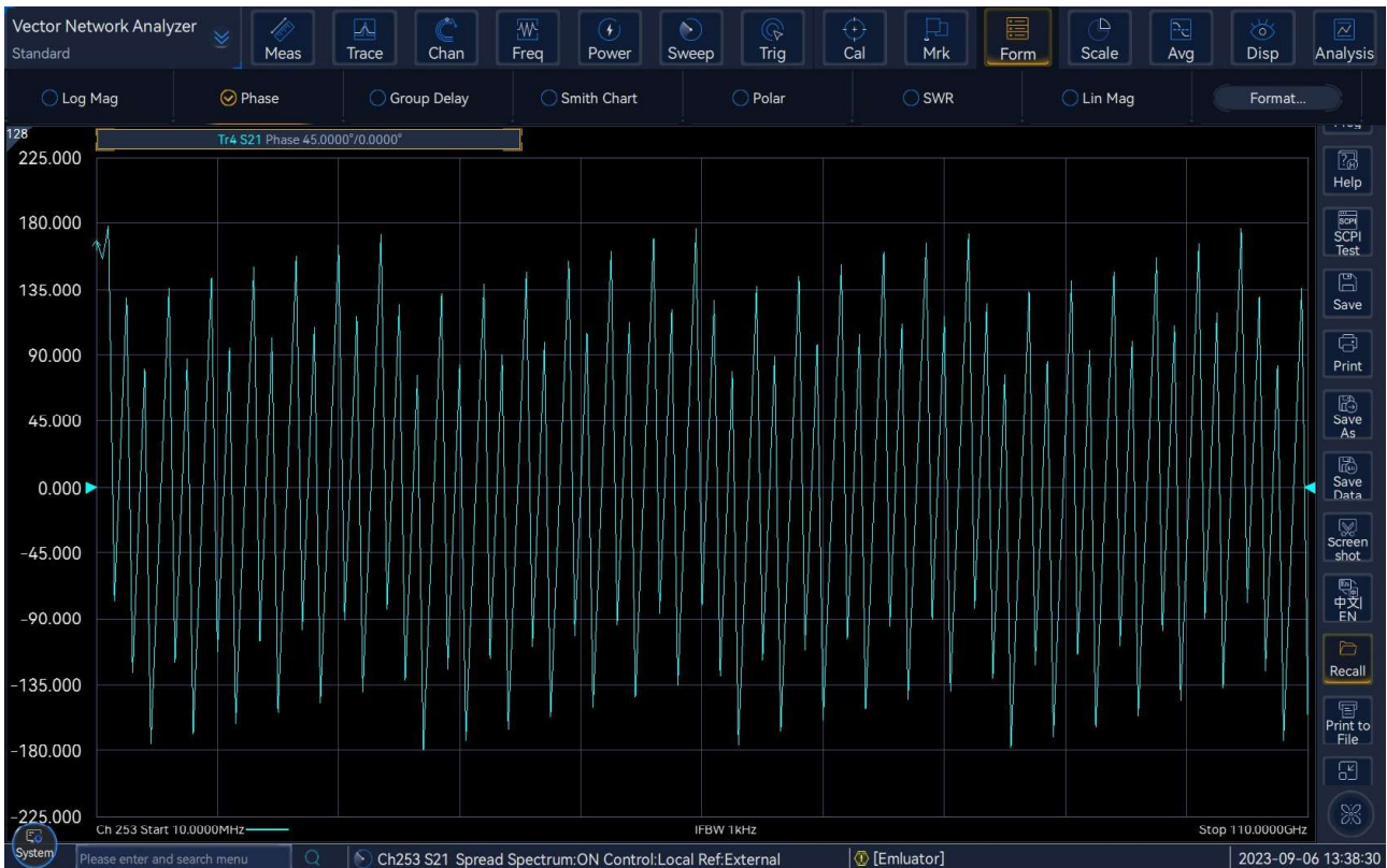
Testing of phase frequency characteristic
