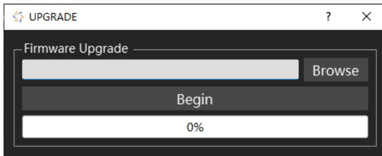
**Note:** Please ensure that line power is constant during the upgrade by using an Uninterruptible Power Supply (UPS), Failure to maintain line power may be cause upgrade failure or instrument damage.
