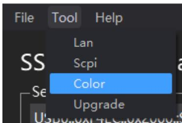
2. The color of RF connectors A-D and the connected RF connectors 1-24 can be configured through the drop-down menu bar. Click Default to restore the default color settings.
