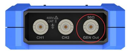
Figure 5-1: Generator Output Ports
