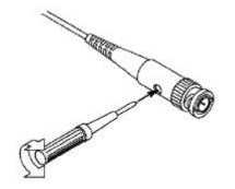
Figure 3-6: Probe Adjustment
