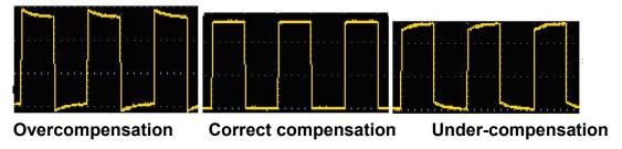
Figure 3-5: Display Waveform of Probe Compensation
