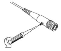
Figure 3-7 Adjust Probe
