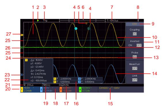
Figure 3-4 Illustrative Drawing of Display Interfaces
