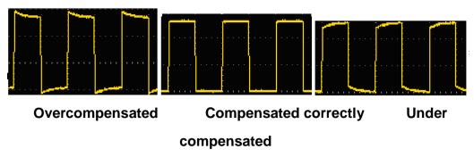
Figure 3-6 Displayed Waveforms of the Probe Compensation
