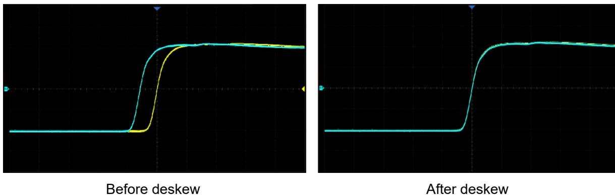
**Note:** When the channel with deskew compensation is the trigger source, the trigger delay indicator does not change as the deskew value changes.
