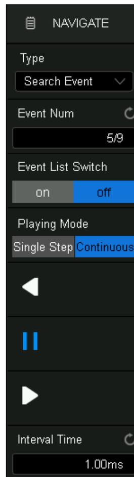
Touch the **Event List Switch** area to turn on or off the list. The list contains time labels for each event. Touching a row in the list automatically jumps to the corresponding event. This operation is equivalent to specifying an event in the **Event Num** area.
