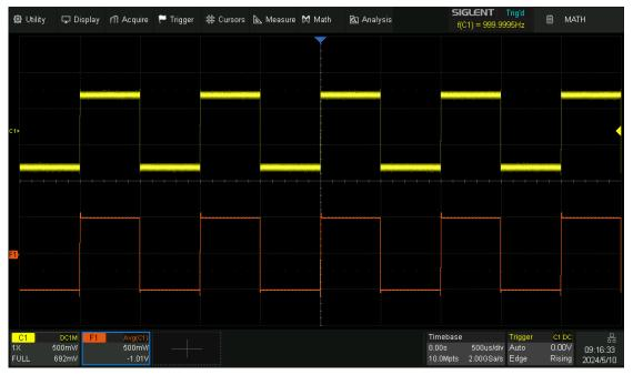
**Note**: Average acquisition is only valid for periodic signals, and it is important to ensure that the waveform is triggering in a stable way when using average mode.
