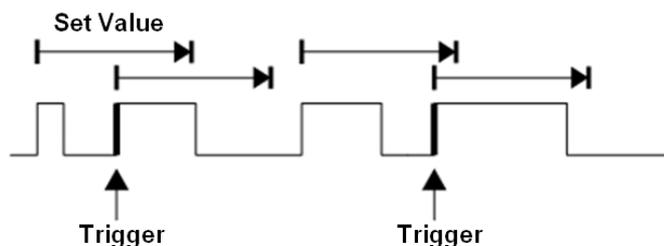
Trigger source, slope (rising, falling), limit range and time value can be set in the trigger dialog box. Holdoff, coupling, and noise reject can be set in the interval trigger, see the sections "Holdoff", "Trigger
