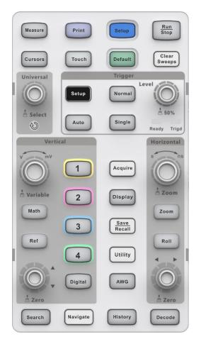
The front panel is designed to operate the basic functins without having to open the software menu. Most of the front panel controls duplicate functionality available through the touch screen display but the operation is more quickly achieved.
