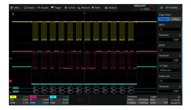
When the CS type is set to Clock Timeout, turn on Cursor, measure the clock idle time between frames as 505  $\mu$ s, and measure the interval between clock pulses as 0.5  $\mu$ s, then set the timeout to a value between 0.5 and 505  $\mu$ s. In this example it is set to 4.5  $\mu$ s:
