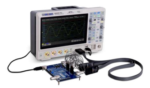
**To connect the logic probe:** Insert the probe, with the correct side facing up, until you hear a "click". **To remove the logic probe:** Depress the buttons on each side of the probe, then pull out it.
