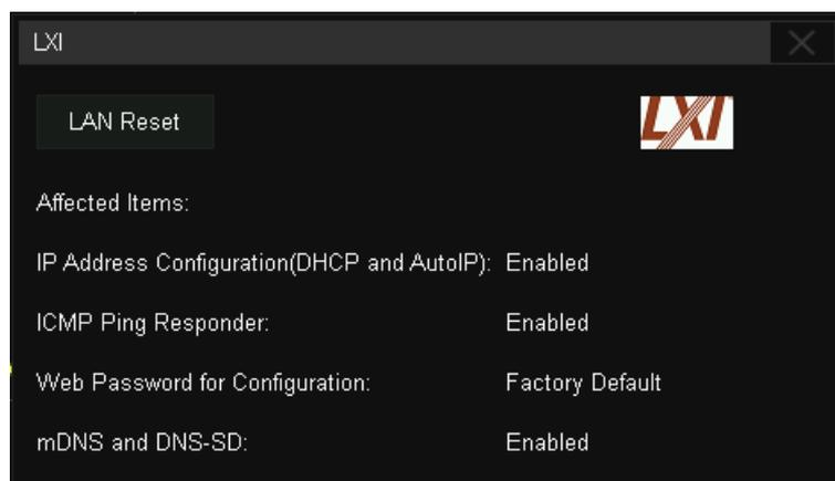
Click **LAN Reset** to restore the LAN defaults to your oscilloscope. It will enable automatic IP, ICMP Ping responder, and Multicast DNS, and reset the webserver password which is set in **Utility** > **Service** > **Web**.
