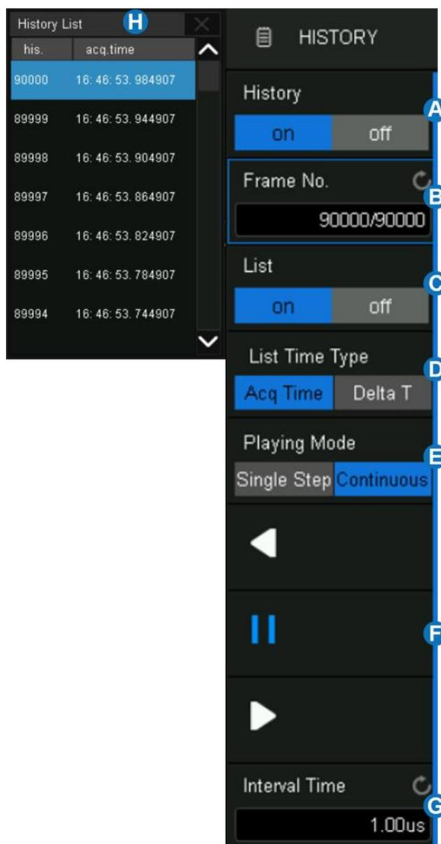
The oscilloscope automatically stores acquired frames. It can store up to 90,000 frames but the number may vary due to the memory depth and timebase settings. Turn on history mode, then the stored frames can be recalled and measured.
