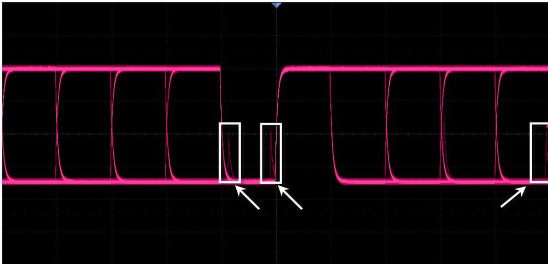
When the display dialog box and persist are off, double-pressing the **Display** button on the front panel can quickly turn on persistence.
