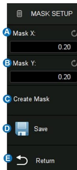
Set the values for **Mask X** and **Mask Y** (in divisions of display graticule), and then perform **Create Mask** to generate the mask. The horizontal and vertical adjustment range is 0.08~4.00 div.
