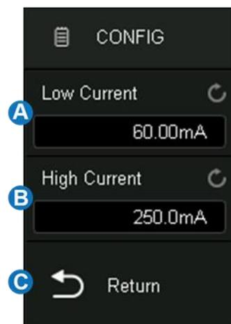
**Note:** low current value and high current value are used to calculate the trigger level and adjust the oscilloscope vertical scale. After the load changes, the current value changes from low to high (or from high to low), and the oscilloscope triggers and performs to measure the transient response stability time.
