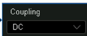
**List:** Sets parameters with more than two options, such as the coupling mode of channels. Touch the parameter region, and then select the expected option from the pop-up list.
