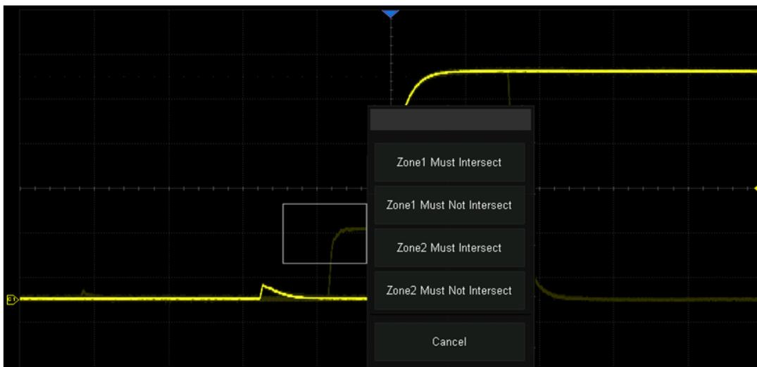
Now, we can accurately capture the exact bus contention waveform:
