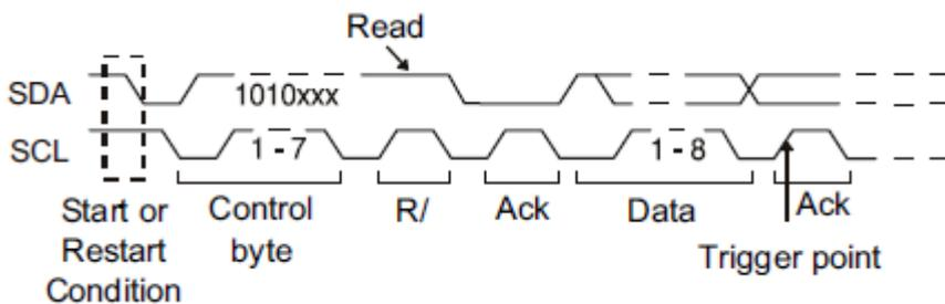
**7 Address & Data** — the oscilloscope will be triggered on read or write frame in 7-bit address mode. Frame (Start: 7-bit address: R/W: Ack) — Data1 and Data2 are set to “0xXX”. If all bits match, then trigger on the Ack bit followed by the R/W bit.
