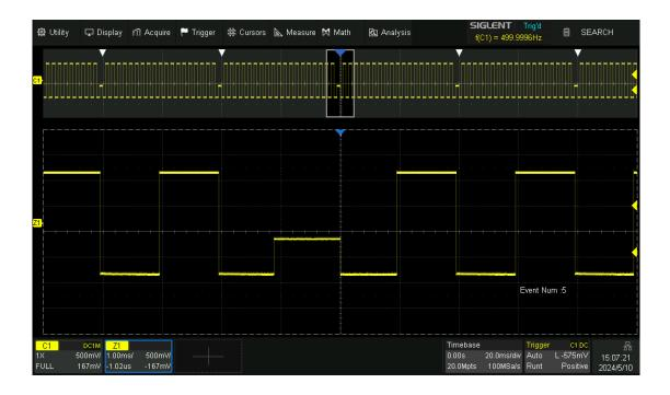
Press the Run/Stop button on the front panel to stop the acquisition, and then follow the steps  $\boxed{\text{Navigate}} > Type$  to select "Search Event". The following figure shows the first dwarf pulse. In this example, the list is enabled and time labels of each event are shown in the list.
