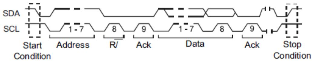
**Restart** — The oscilloscope will be triggered when another “Start” occurs before a “Stop”.
