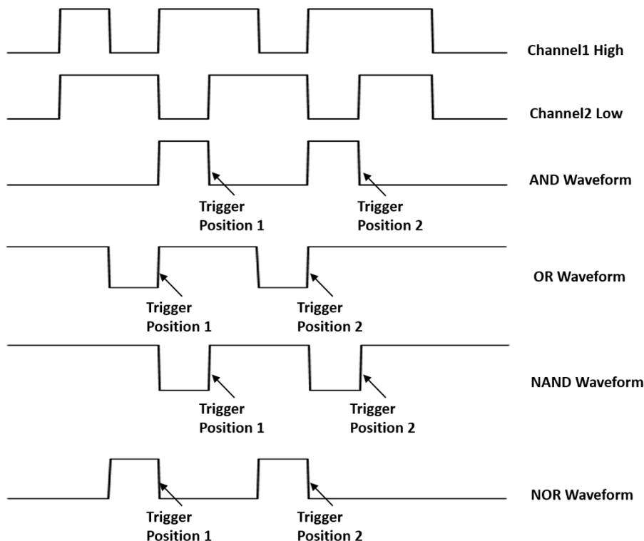
Logic (AND, OR, NAND, NOR), source, limit range, and time value can be set in the trigger dialog box. When the logic is "OR" or "NAND", the setting of the time limit is invalid.
