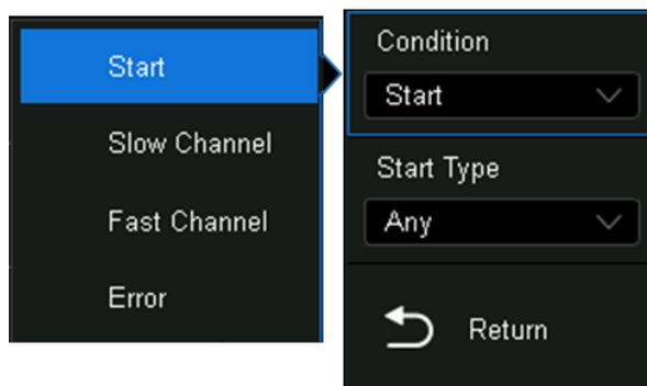
**Start** — the oscilloscope will be triggered on the start of message (after 56 synchronization ticks). You can select the type of the message: Fast Channel Message, Slow Channel Message or any.
