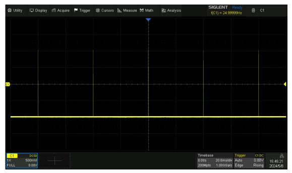
In normal mode, 5 pulses can be obtained on the screen with the sample rate of 1 GSa/s at the maximum memory depth.
