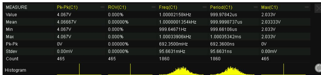
Touch the histogram area of a parameter to enlarge it for details. You can move the large histogram window position around the display by dragging. Touch the histogram of another parameter to switch to the corresponding enlarged histogram.
