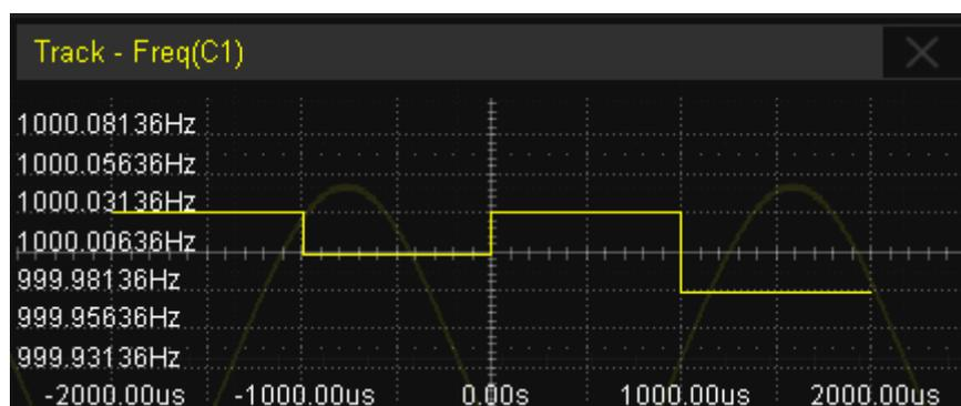
1000 is the default upper limit of the statistic number in a frame, which means the values exceeding the limit will not be shown in the track plot.
