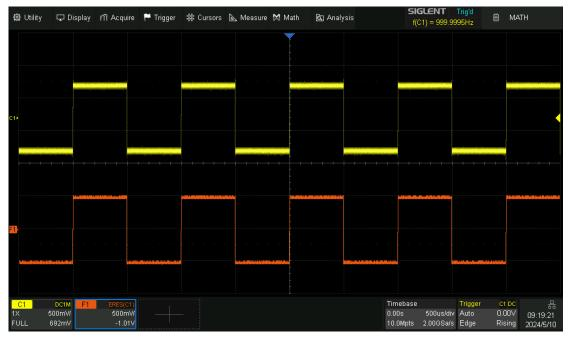
ERES operation does not require the signal to be periodic, nor does it require stable triggering, but due to the digital filtering, the system bandwidth of the oscilloscope will degrade when acquiring data in ERES mode. The higher the enhanced bits, the lower the bandwidth. The following table shows the relationship between ERES bits and bandwidth:
