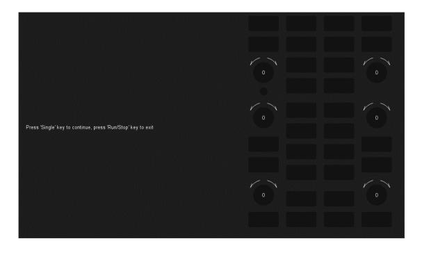
Press the Single button and the first LED on the front panel will light. The corresponding position of the key on the screen will also change color. Press the Single button to check the next button. Press the Single button consecutively until all the backlights are tested.
