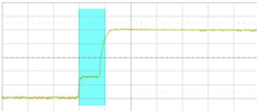
With a simple edge trigger, it is unlikely to trigger consistently on this anomaly. Thanks to the high waveform update rate of the SDS2000X Plus, we can confirm there is bus contention happening by enabling the persistence display, as shown in the figure below:
