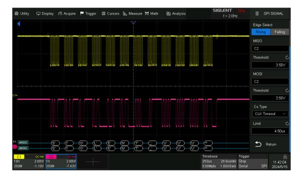
If the data width is set to be greater than 8-bits (such as 16-bits), measure the clock idle time between 8-bit data packets as  $5.05 \ \mu$ s, and then set the timeout time to a value between  $5.05 \ and \ 505 \ \mu$ s. In this example, it is set to 80  $\mu$ s:
