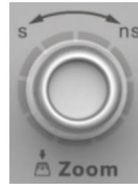
When the Zoom function is on, the waveform area is divided into upper and lower parts. The area of about 1/3 height above is the main window, and the area of about 2/3 height below is the zoom window. Touch a window to activate it.
