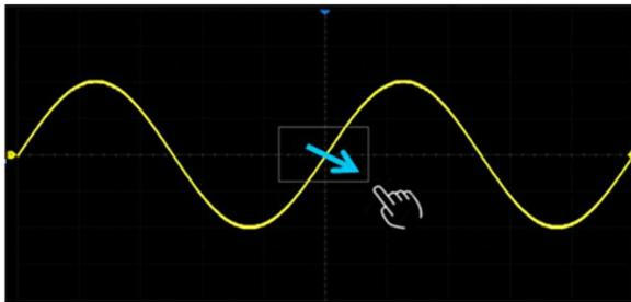
Draw a rectangular box to create a zone or a histogram region. At the beginning of the gesture keep the angle close to  $45^\circ$  so it can be recognized as the drawing box gesture
