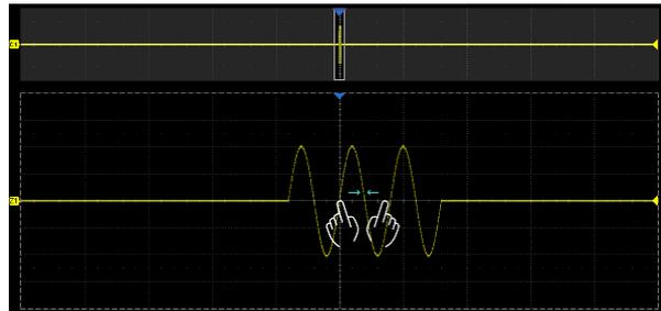
Adjust the horizontal scale of the Zoom window by horizontal pinch and spread in the zoom area of the main window or in the Zoom window
