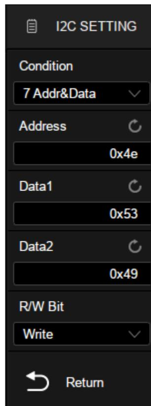
**Data Length** — The data length range is 1 to 12 bytes. When the SDA data length is equal to the value of the Data Length setting and the address length is the same as the set value, the oscilloscope will be triggered.
