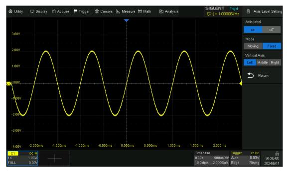
Turn on axis lable, the axis mode is Fixed, and position of the axis label is on the left side of the screen
