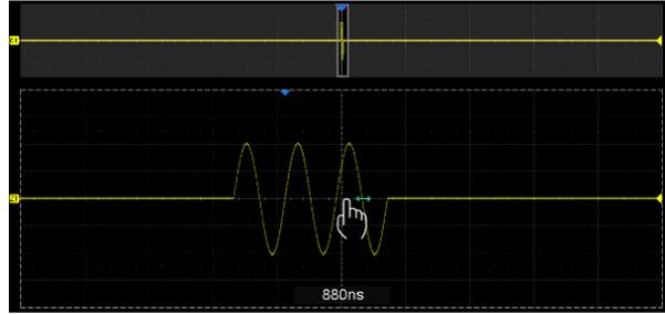
Adjust the horizontal position of the zoom area by dragging left and right in the zoom area of the main window or waveform in Zoom window
