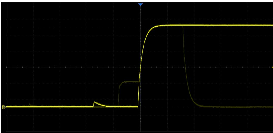
In this case, the zone trigger is a quick and simple way to capture the interesting waveform. Enable the zone trigger, and draw a box to intersect with the bus contention part, as shown in the figure below:
