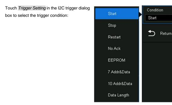
**Start** — The oscilloscope will be triggered when the SDA line transitions from high to low while the SCL is high.
