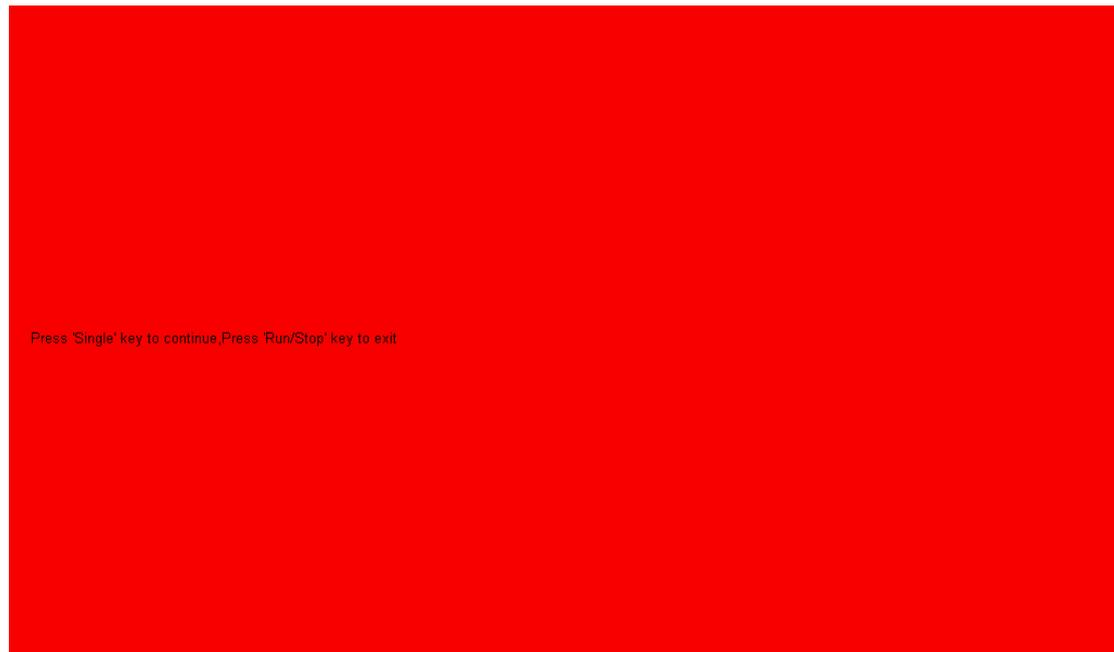
Press the **Single** button to switch to green and blue display mode. Observe whether there is any color distortion, bad pixel or scratch on the screen.
