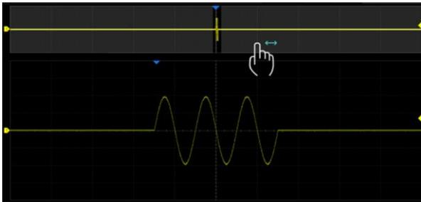
Adjust the horizontal position of the waveform by dragging left and right in the gray area of the main window
