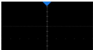
**Trigger Delay Indicator** locates where the waveform triggers on the horizontal axis... When the trigger position is outside the screen, the direction of the triangle changes to point outside the screen.
