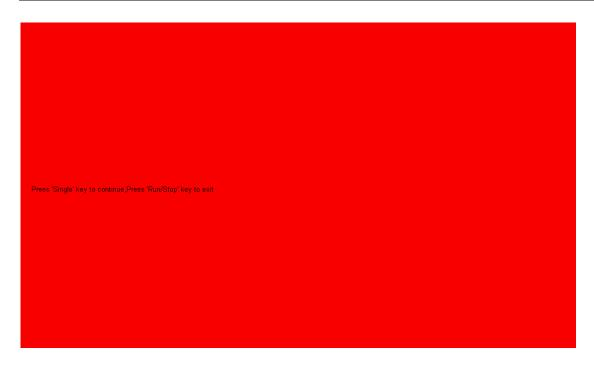
Press the Single button to switch to green and blue display mode. Observe whether there is any color distortion, bad pixel or scratch on the screen.
