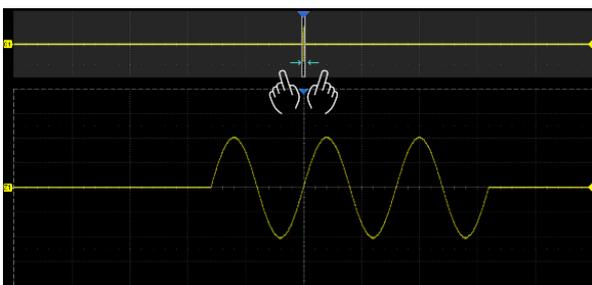
Adjust the horizontal scale of the main window by pinch and spread in the gray area of the main window
