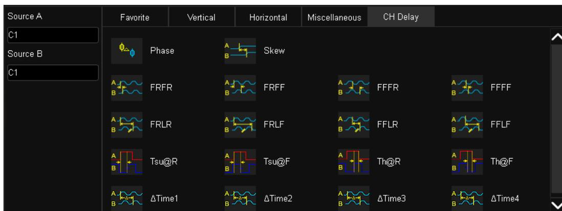
In the parameter selection area, the channel corresponding to **Source A** is specified first, and then the channel corresponding to **Source B**. Finally, the measurement parameter is selected. For example, to activate the skew between C1 and C2, you can follow the following steps:
