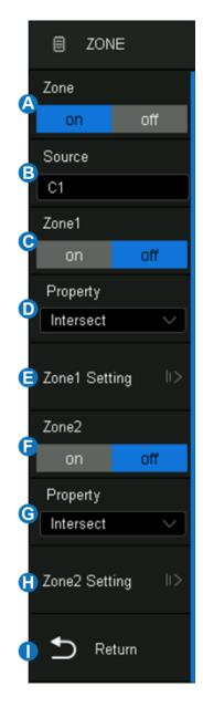
The zones can be created and moved by gestures or by setting *Zone* > *Zone Setting* in the dialog box. The color of the zone's outline is consistent with the color of the specified source (Channel 1 = Yellow, etc...).
