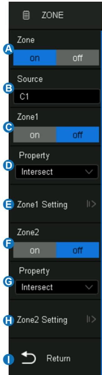
The zones can be created and moved by gestures or by setting *Zone* > *Zone Setting* in the dialog box. The color of the zone's outline is consistent with the color of the specified source (Channel 1 = Yellow, etc...).
