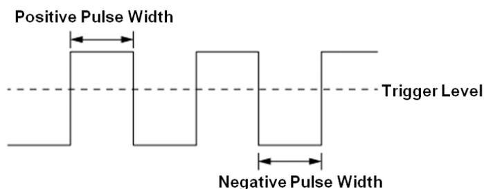
**Less than a time value ( $\leq$ )** — Trigger when the positive or negative pulse time of the input signal is lower than the specified time value. Below is an example of trigger condition is set to positive pulse width < 100ns
