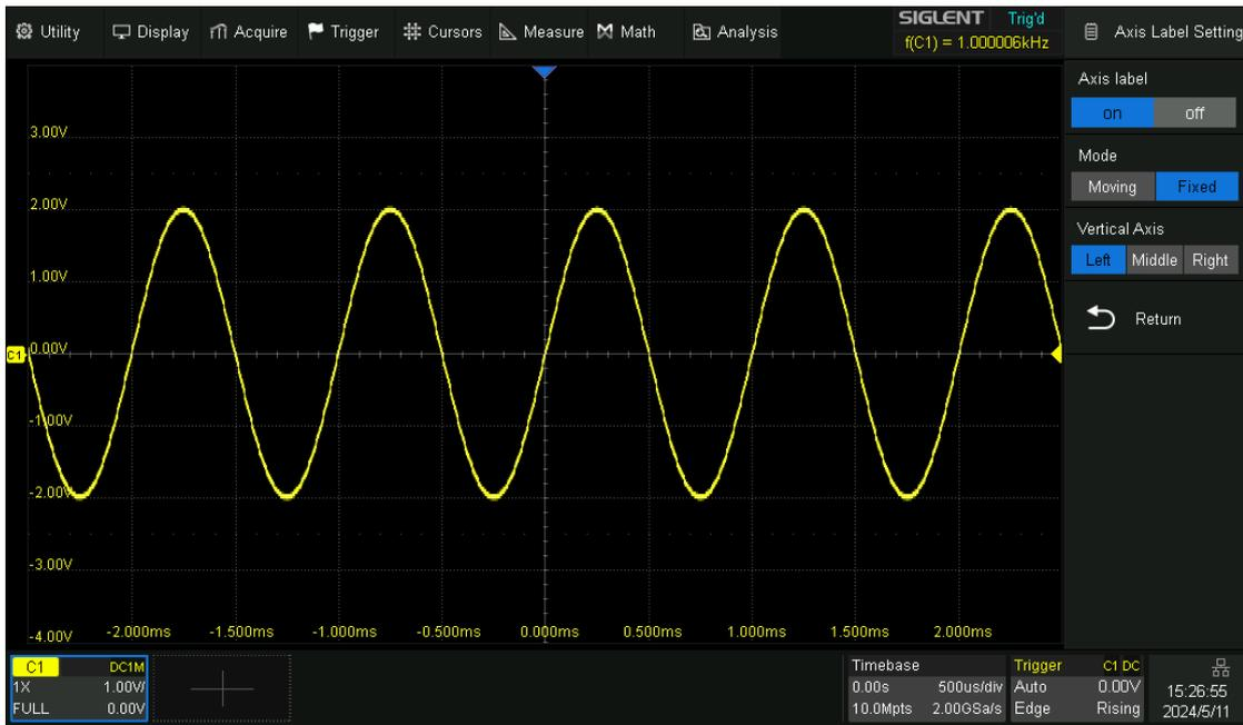
Turn on axis label, the axis mode is Fixed, and position of the axis label is on the left side of the screen
