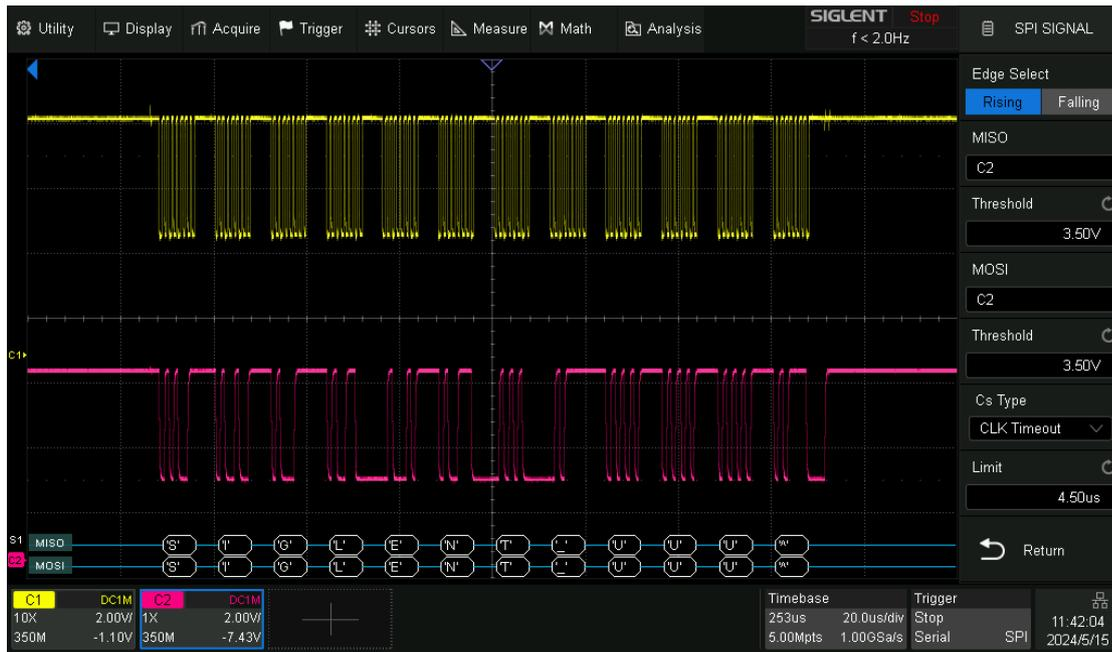
If the data width is set to be greater than 8-bits (such as 16-bits), measure the clock idle time between 8-bit data packets as 5.05  $\mu$ s, and then set the timeout time to a value between 5.05 and 505  $\mu$ s. In this example, it is set to 80  $\mu$ s:
