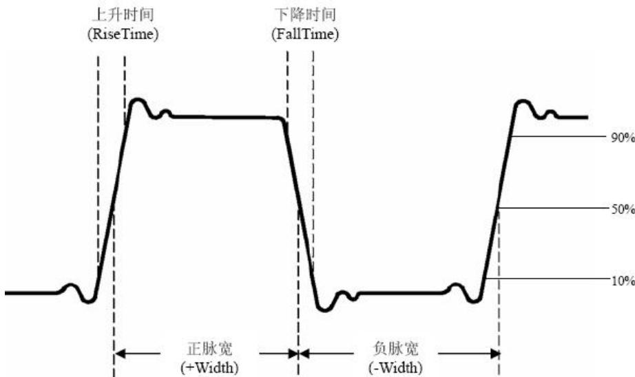
**RiseTime:** The time span for signal amplitude rise from 10% to 90%, judged by the rising edge of its first pulse.
