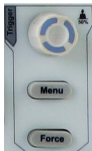
Figure 3- 13 Trigger Control Zone
