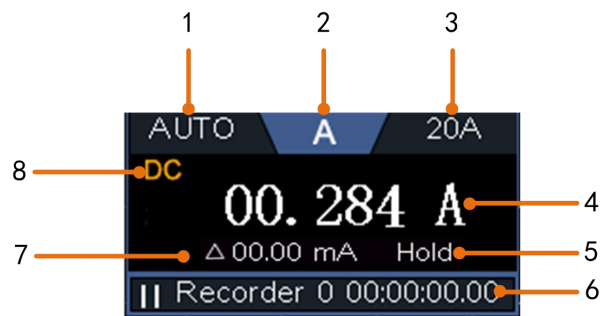
Figure 6-3 Multimeter Information Window
