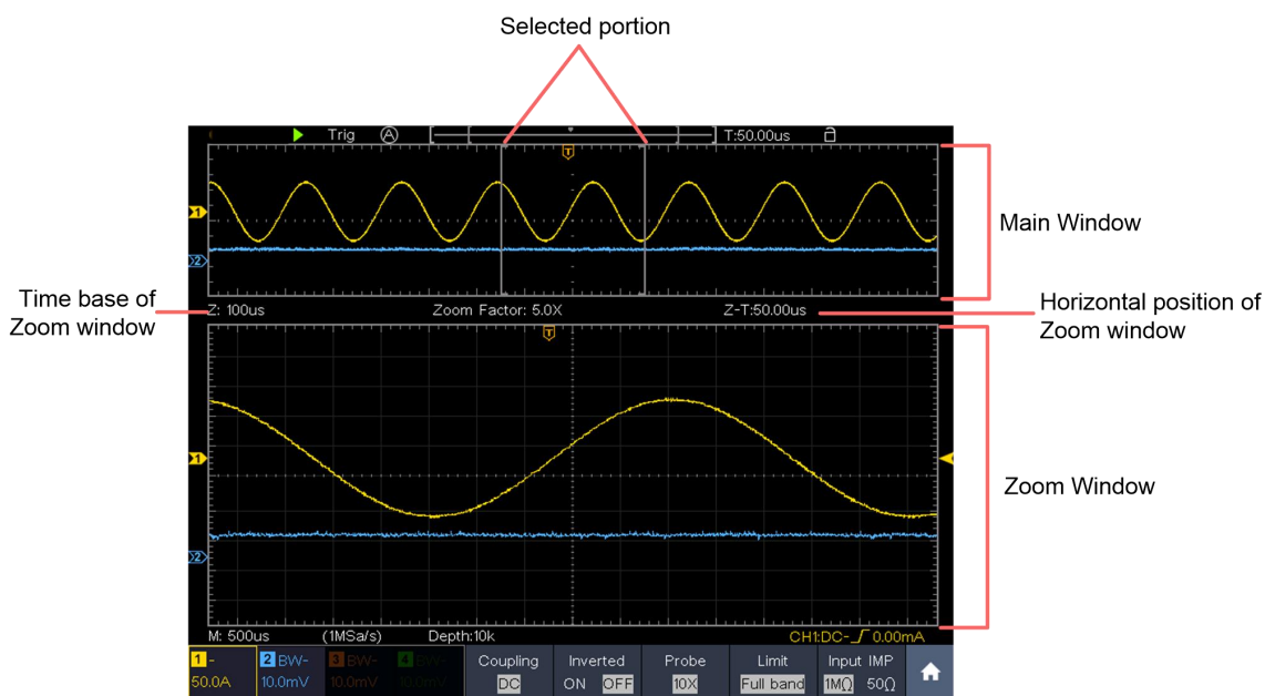
Figure 4- 8 Waveform Horizontal Zooming Mode
