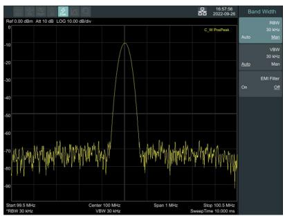
Figure 4-9 Set frequency span
