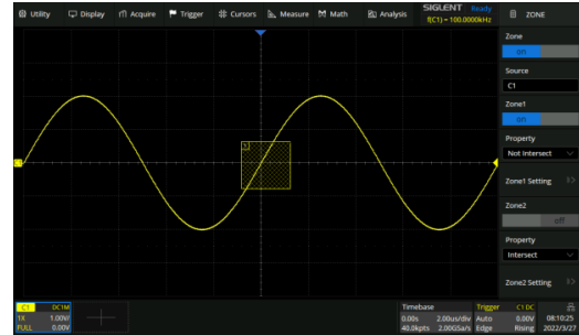
Select C1 as the source, turn on zone1, and set the property as "Not Intersect"
