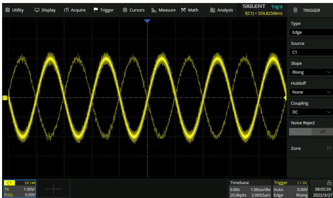
Noise Reject = Off
