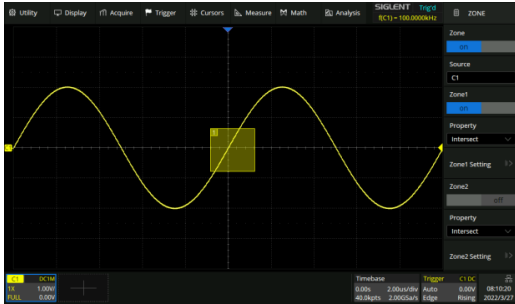
Select C1 as the source, turn on zone1, and set the property as "Intersect"
