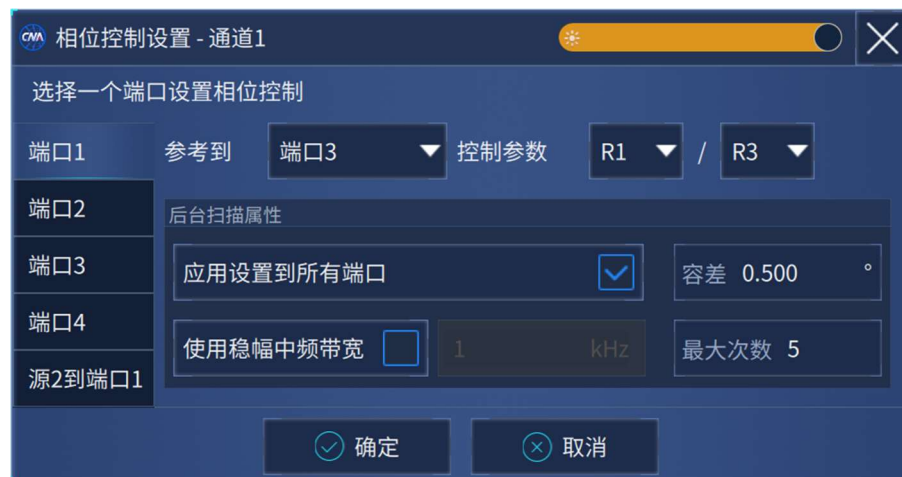
Figure 4. 18 Setting to phase sweep
