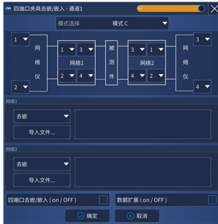
Figure 7.46 4-port fixture de-embedding/embedding interface
