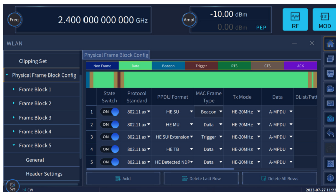
WLAN Physical Frame Block Interface
