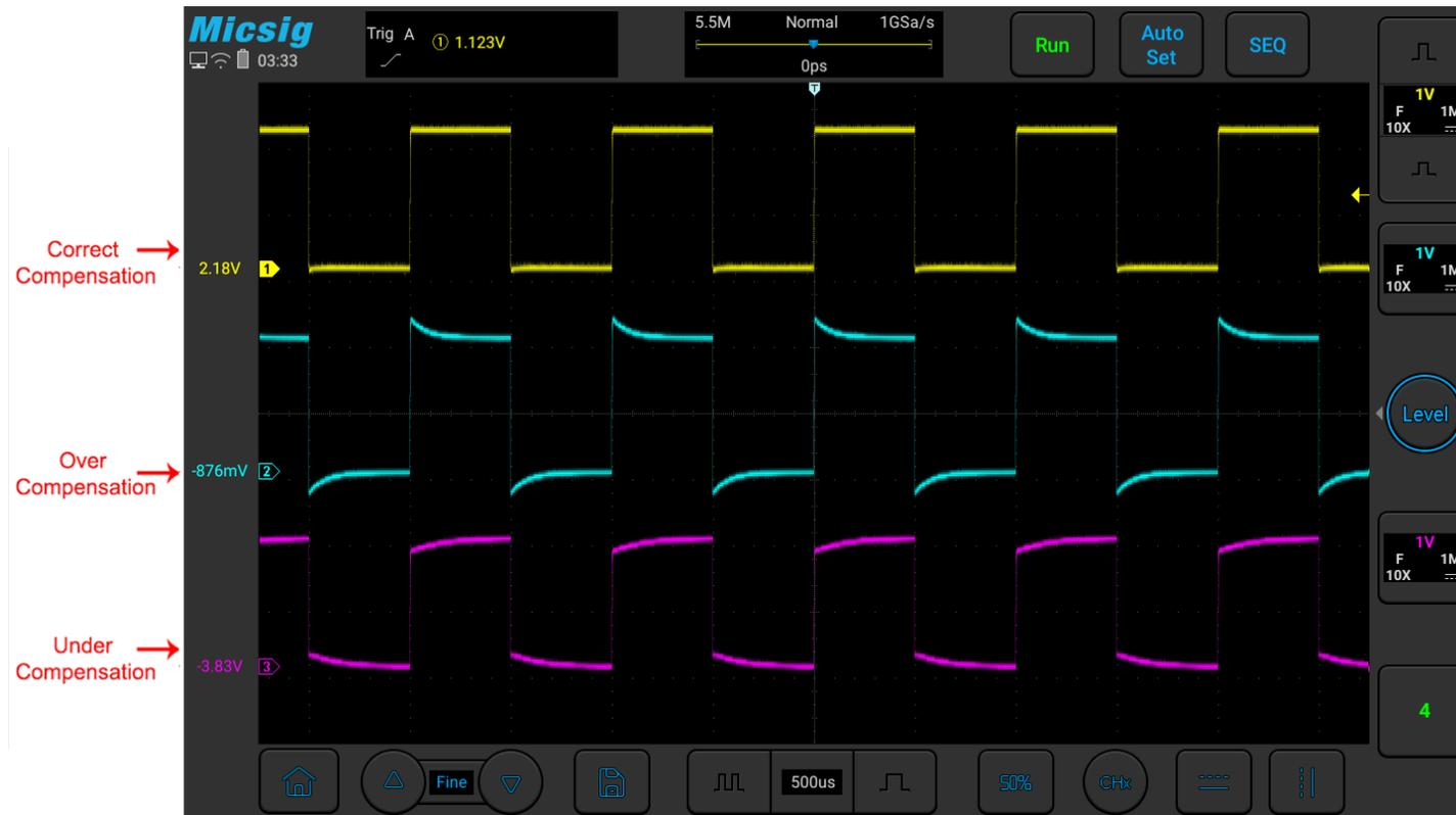
Figure 2-15 Probe Compensation
