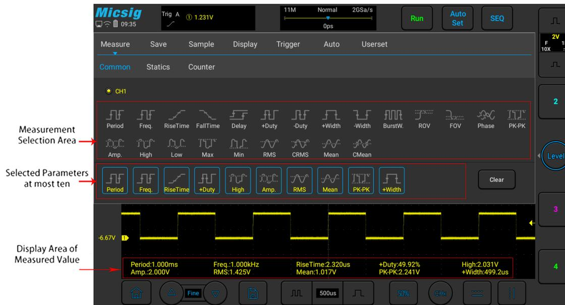
Figure 6-1 Automatic Measurement Menu
