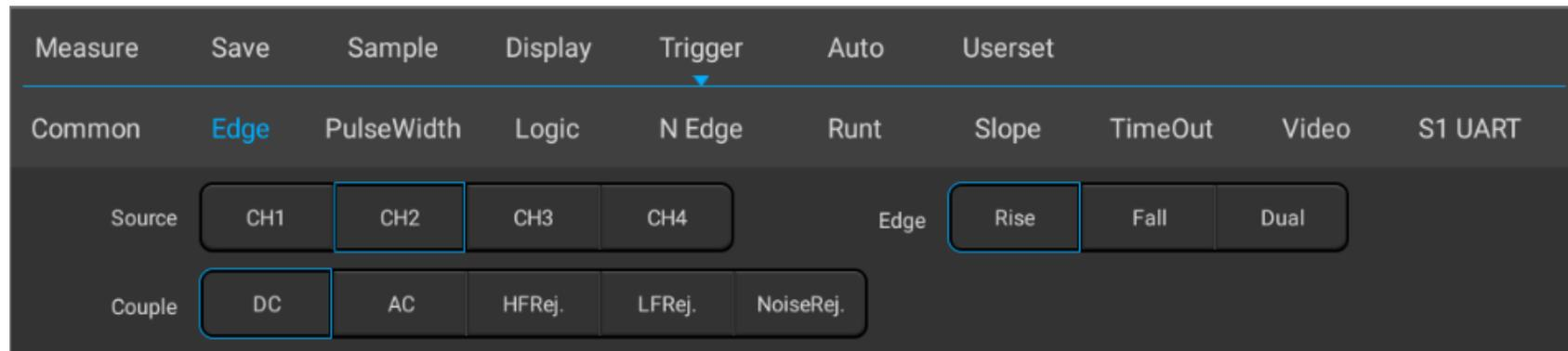
Figure 5-12 Edge Trigger Setting Menu
