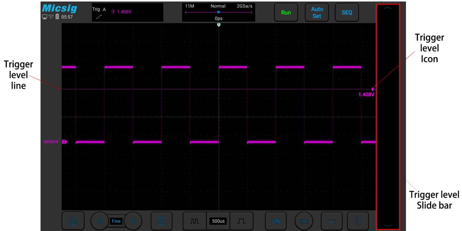
Figure 5-8 Trigger Level
