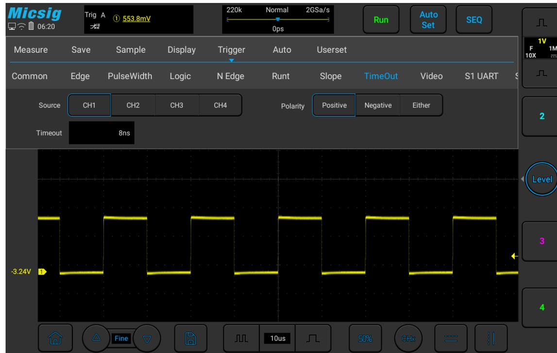
Figure 5-29 Time-out Trigger
