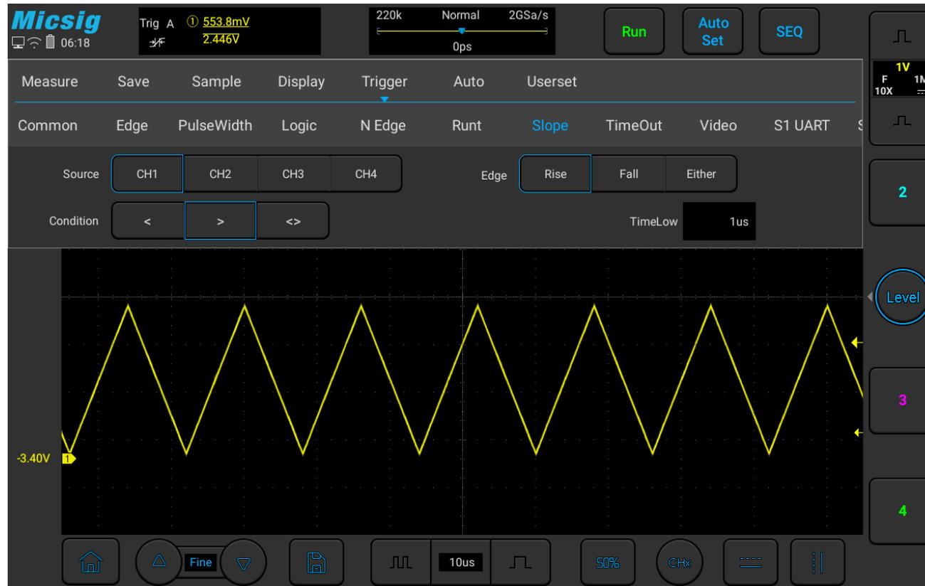
Figure 5-27 Slope Trigger Setting Menu
