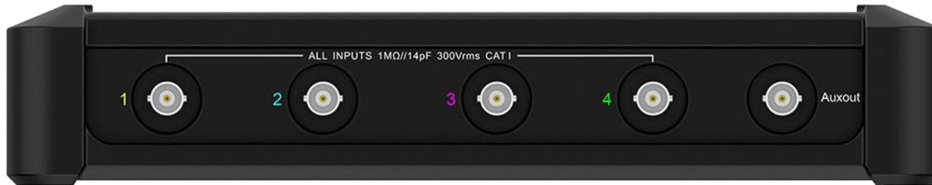
Figure 2-4 Top Panel of Tablet Oscilloscope
