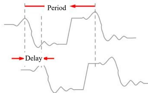
Figure 6-6 Phase Measurement Schematics
