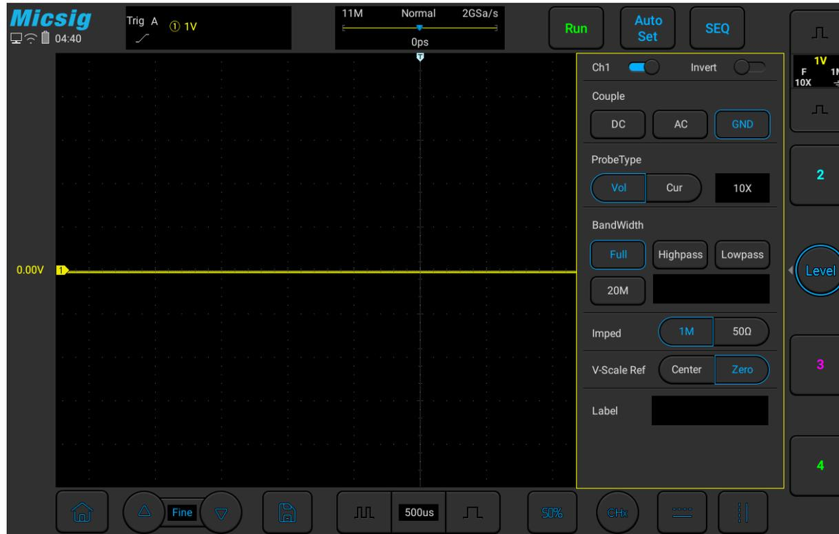
Figure 4-9 GND Coupling
