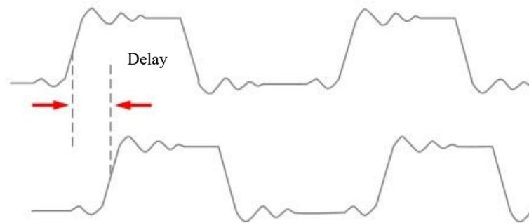
Figure 6-5 Delay Measurement Schematics
