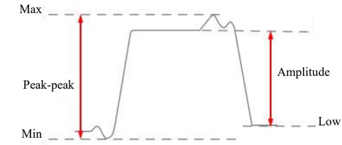
Figure 6-7 Voltage Measurement
