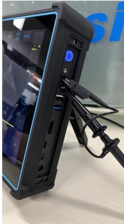
Figure 2-14 Probe Connection
