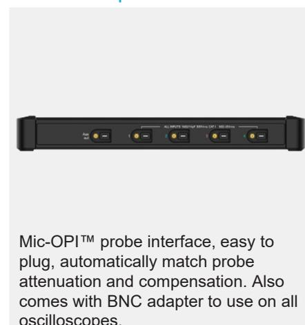
Mic-OPI™ probe interface, easy to plug, automatically match probe attenuation and compensation. Also comes with BNC adapter to use on all oscilloscopes.
