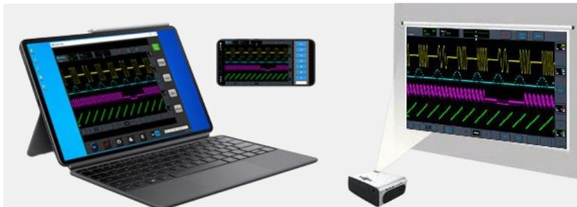
Support remote control via PC, mobile app, and HDMI screen projection. Support SCPI programming commands, helping engineers to conduct tests more flexibly and efficiently.
