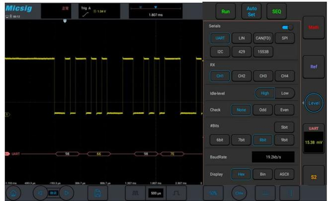
▲ Serial bus decoding and analysis
