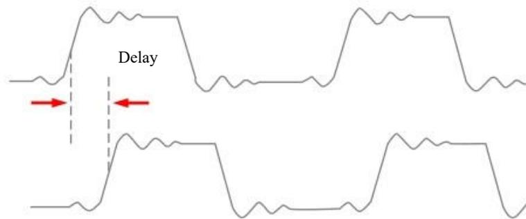
Figure 6-5 Delay Measurement Schematics
