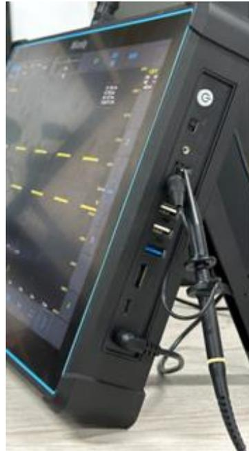
Figure 2-13 Probe Connection
