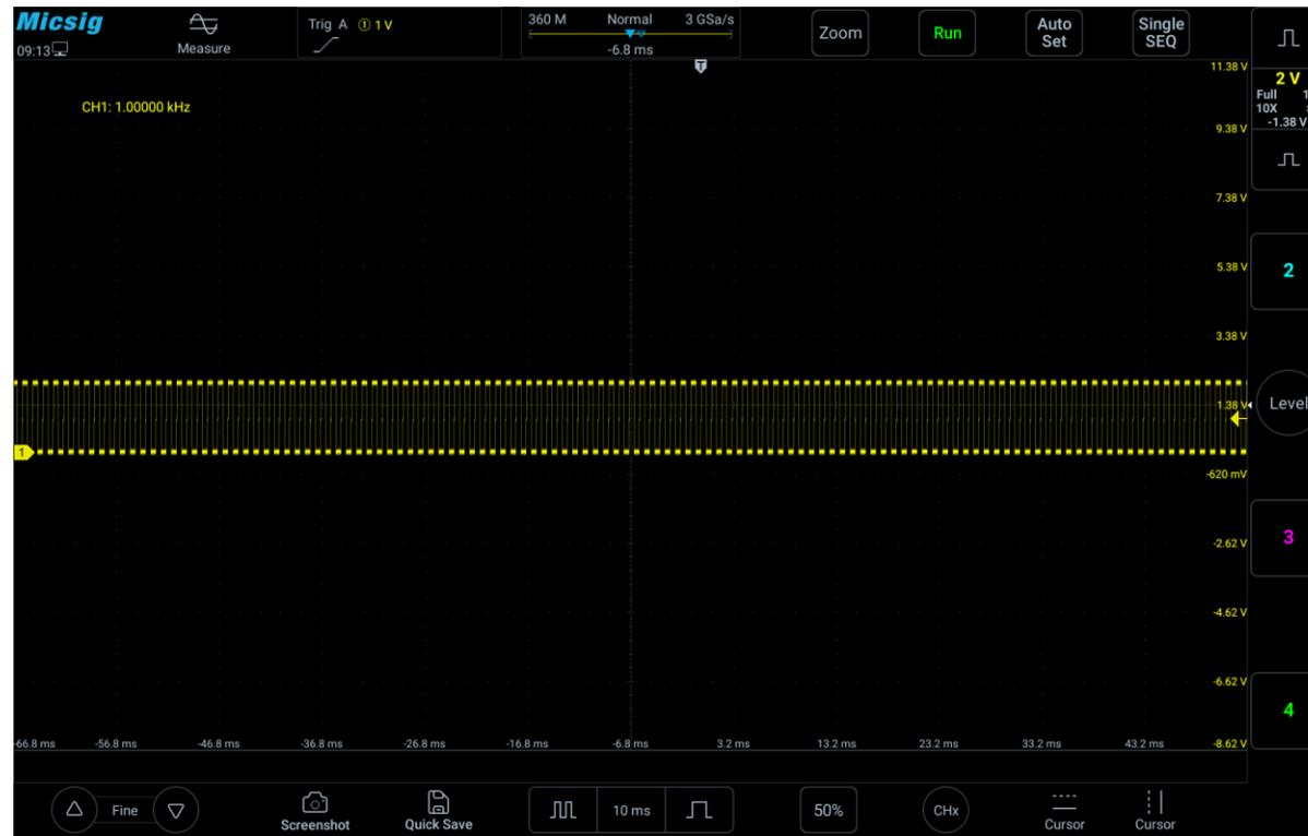
Figure 6-15 Frequency Meter Measurement
