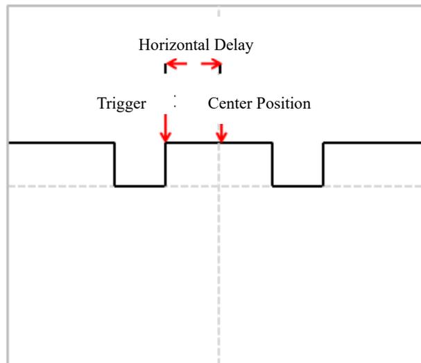
Figure 5-7 Horizontal Delay
