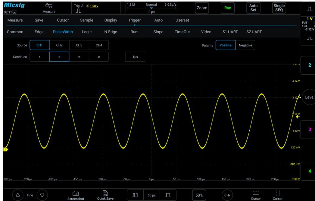
Figure 5-14 Pulse Width Trigger Setting Menu
