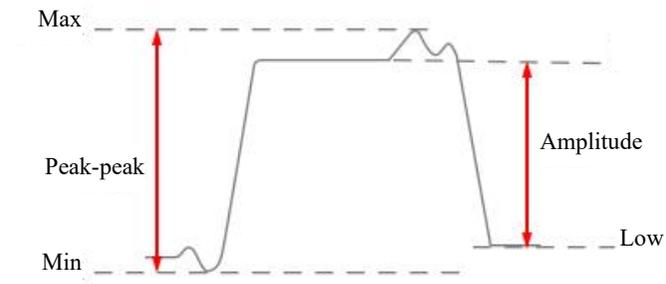
Figure 6-7 Voltage Measurement
