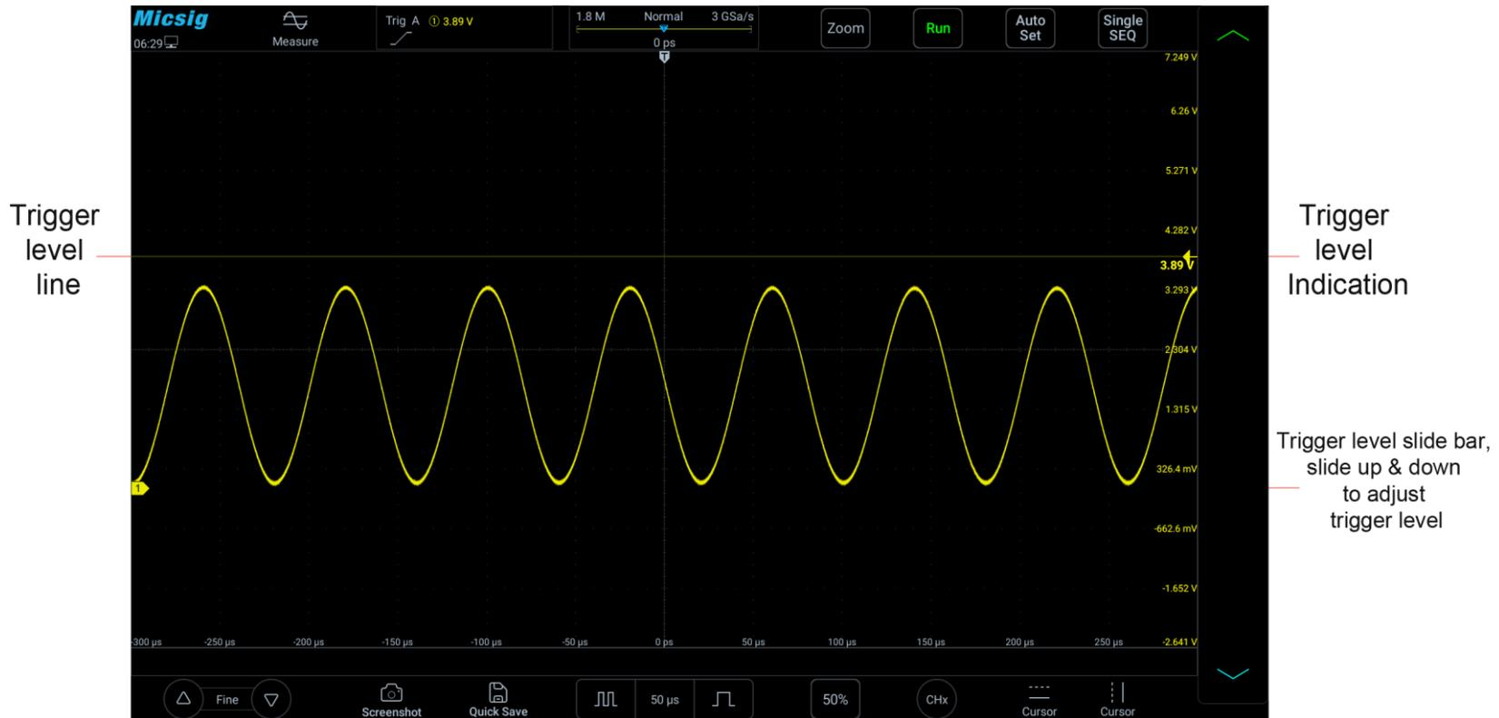
Figure 5-8 Trigger Level
