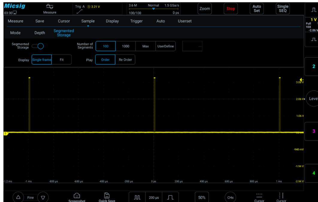
Figure 10-11 Segmented storage waveform acquisition
