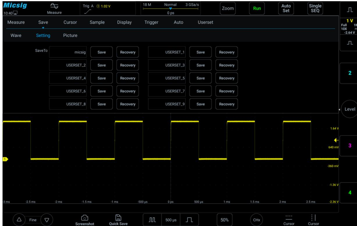
Figure 7-7 oscilloscope setting save
