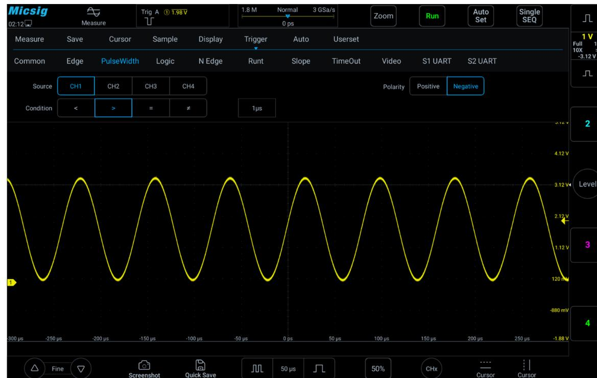
Figure 5-15 Negative Polarity Pulse Level Flip
