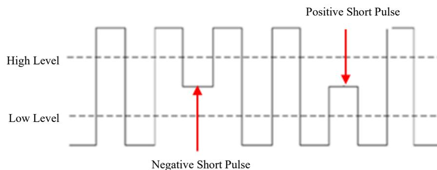
Figure 5-24 Runt Trigger
