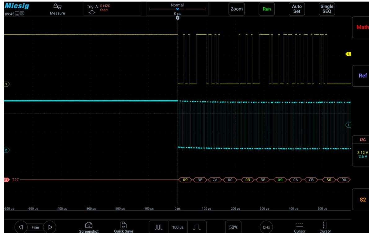
Figure 11-24 I<sup>2</sup>C Graphic Interface
