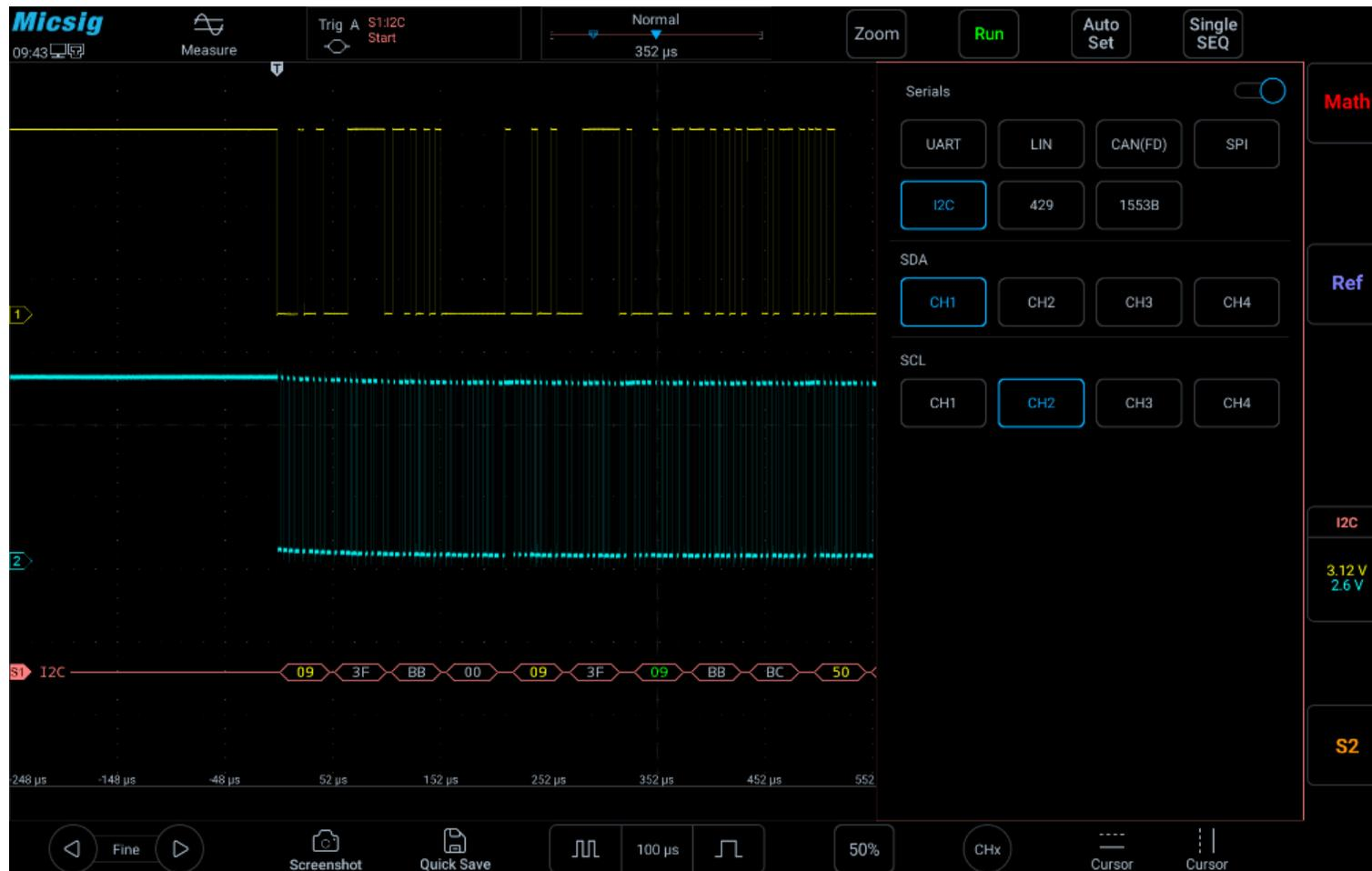
Figure 11-22 I<sup>2</sup>C Bus Configuration Menu
