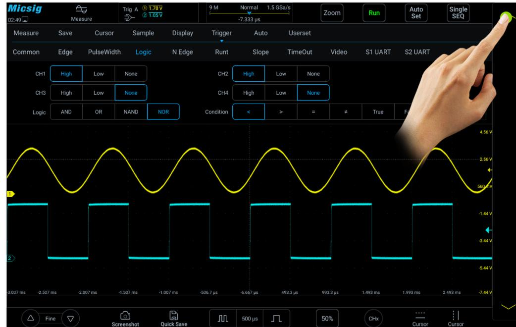
Figure 5-22 Trigger Level Adjustment
