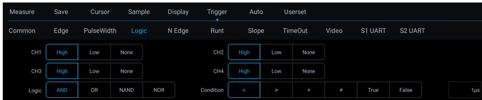
Figure 5-21 Logic Trigger Setting Menu
