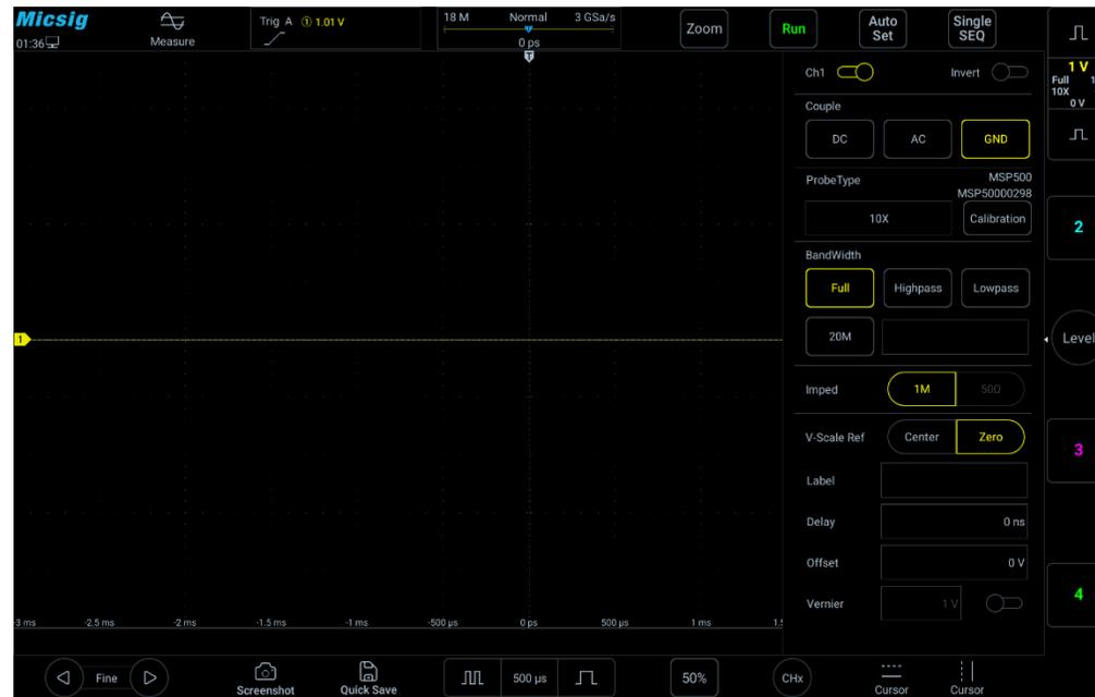
Figure 4-9 GND Coupling
