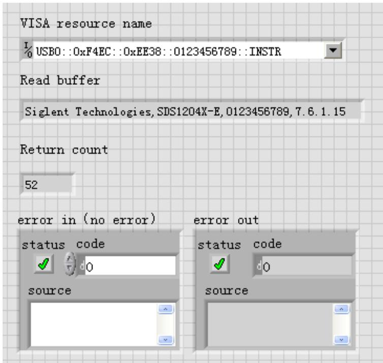
In this example, the VI opens a VISA session to a USBTMC device, writes a command to the device, and reads back the response. After all communication is complete, the VI closes the VISA session.
