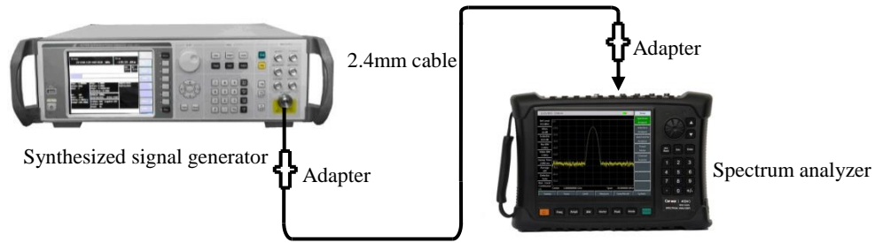
Fig. 4-1 Schematic Diagram of Connection of Signal Generator and Spectrum Analyzer
