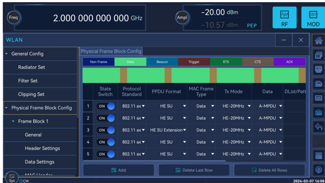
WLAN physical frame block configuration interface
