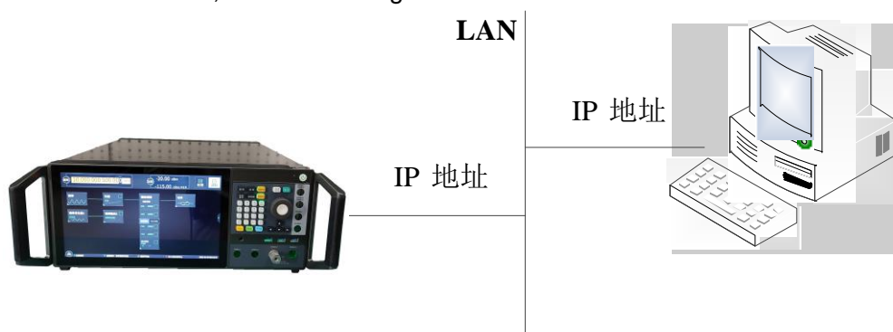
Figure 2.13 LAN interface connection
