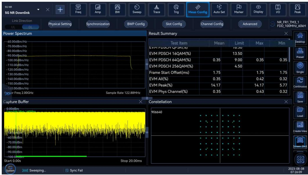
FR1-TM3\_1\_FDD\_100MHz\_60kHz measured value
