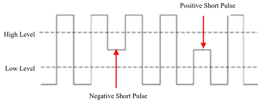
Figure 6-24 Runt Trigger
