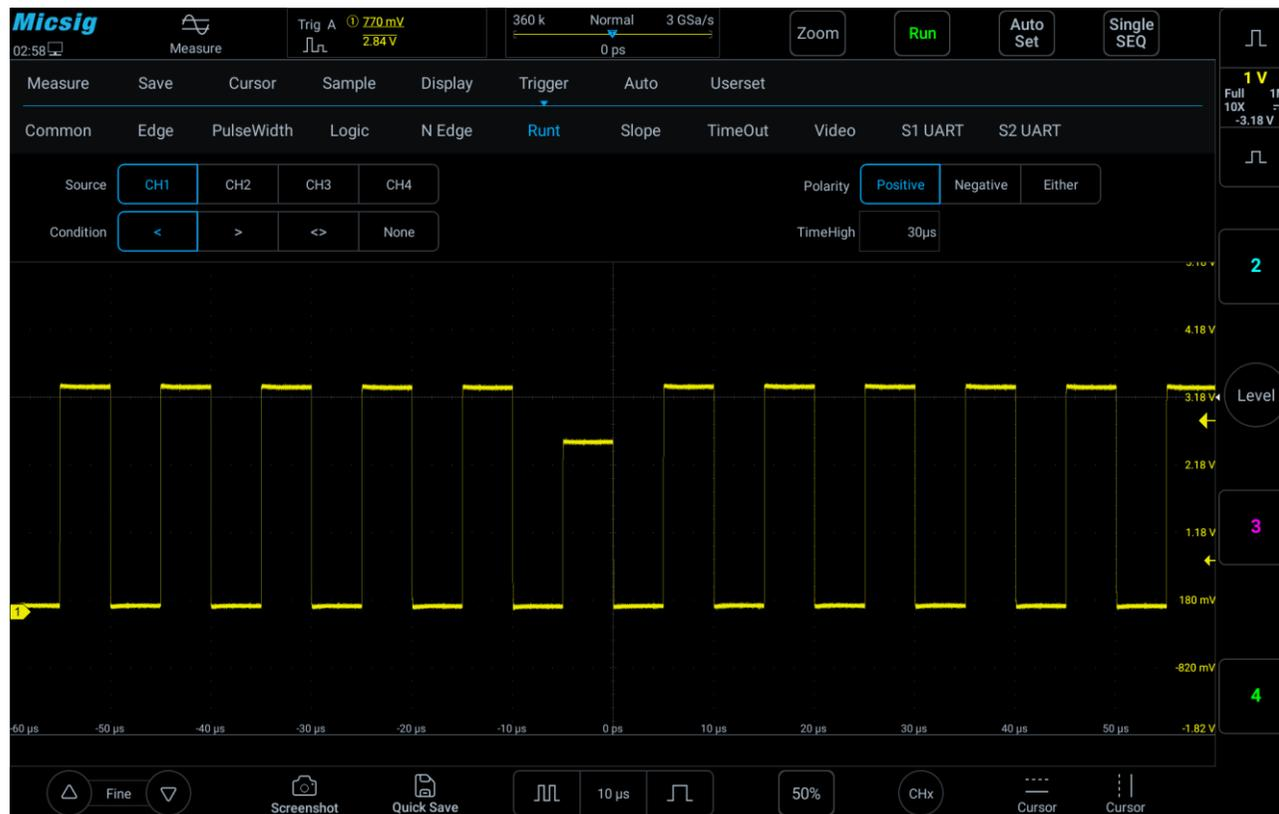
Figure 6-25 Runt Trigger Setting Menu
