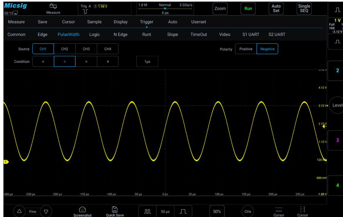
Figure 6-15 Negative Polarity Pulse Level Flip
