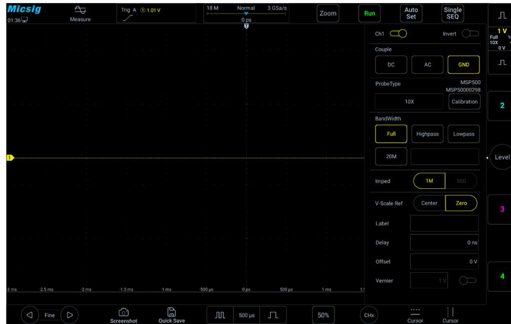
Figure 5-9 GND Coupling
