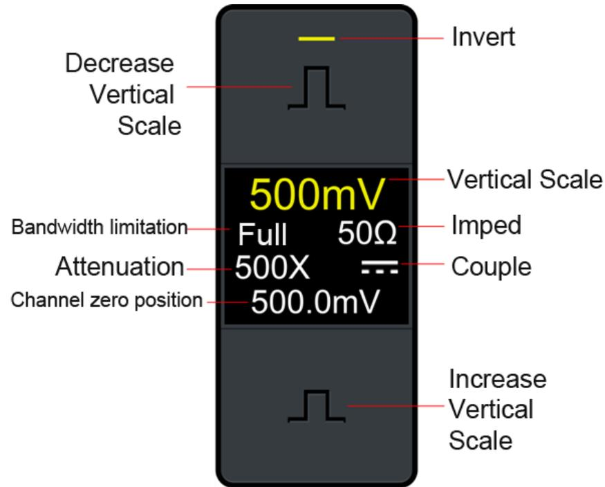
Figure 5-3 Channel Display Interface
