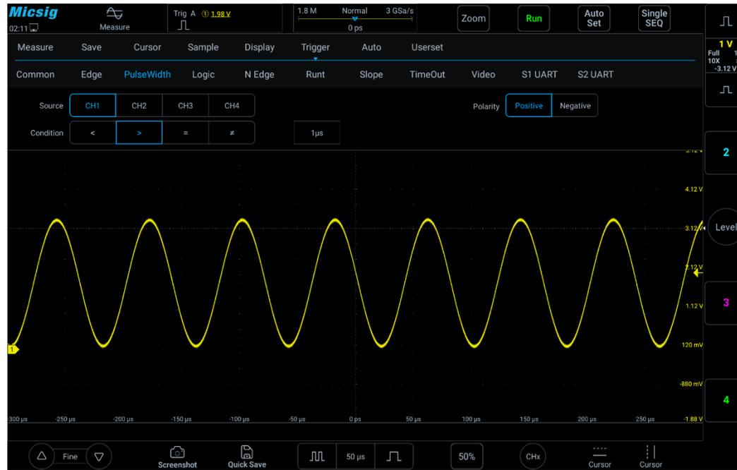
Figure 6-14 Pulse Width Trigger Setting Menu
