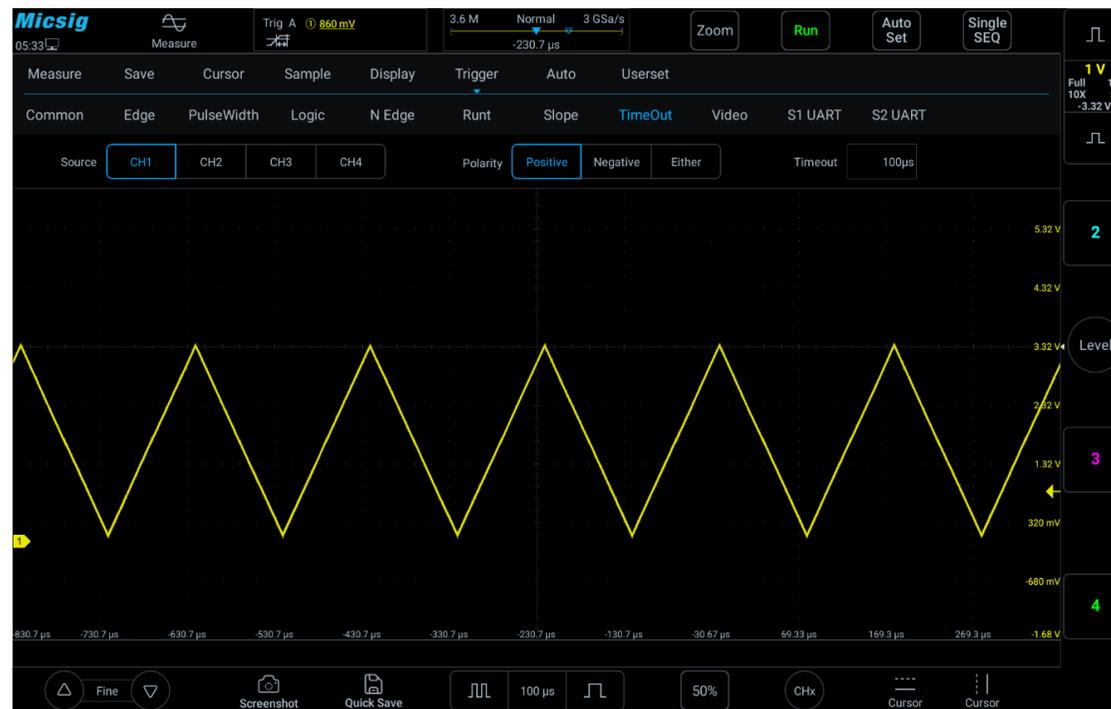
Figure 6-29 Time-out Trigger
