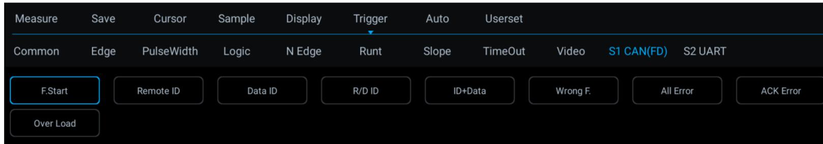
Figure 12-15 CAN FD Trigger Mode Configuration Menu
