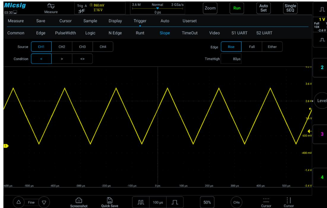
Figure 6-27 Slope Trigger Setting Menu
