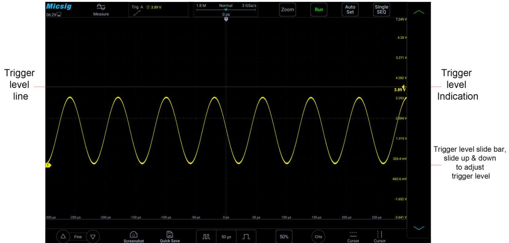
Figure 6-8 Trigger Level
