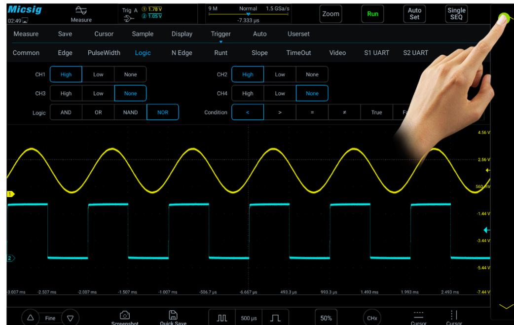
Figure 6-22 Trigger Level Adjustment
