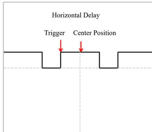
Figure 6-7 Horizontal Delay
