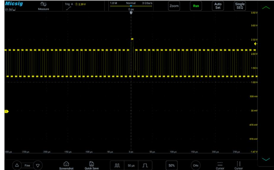
Figure 6-4 Abnormal Signal Captured by Setting Trigger Level
