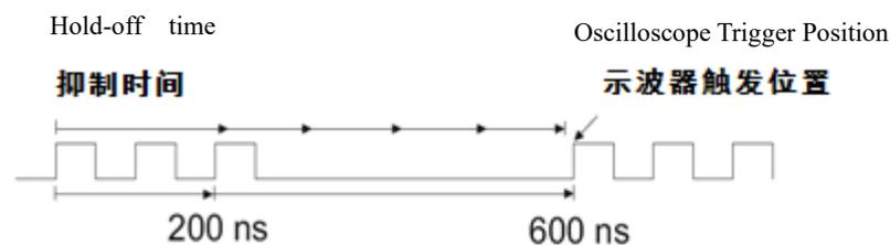
Figure 6-10 Trigger Hold-Off Time
