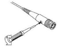
Figure 3-6: Probe Adjustment
