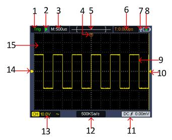
Figure 3-3: Oscilloscope Interface
