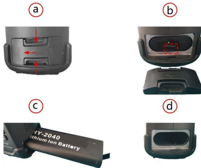
Fig.3.6 1433 series signal generator battery replacement
