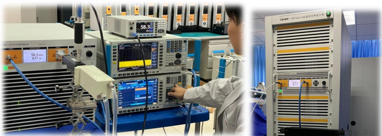
6GHz-18GHz, 650W(up)/ 1GHz-2GHz, 14kW(right)
